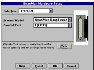
Change the hardware settings for the ScanMan scanner, if necessary, in the Hardware Setup dialog box. The Hardware Setup command button in the ScanMan Options dialog box displays the ScanMan Hardware Setup dialog box. From this box, you can change hardware settings for ScanMan.
